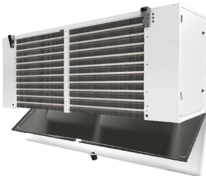
In the CUBIC Vario unit, melting ice and condensation water from the heat exchanger lands in the inner tray and passes from there to the drain. As the channel of the inner tray features an increased gradient, it allows condensation water to drain off more effectively. Ice formation in the tray caused by accumulated condense water is minimized allowing defrosting time to be reduced and results in energy savings.
