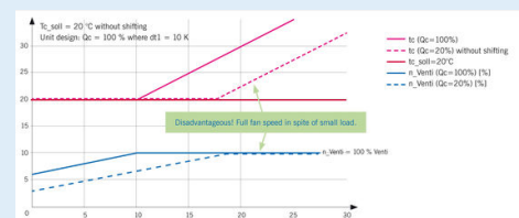
Temperature shifting for reducing the fan speed in summer and at low refrigerating load
