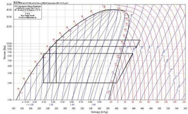
Figure 2: Three refrigerant systems with the same evaporation temperature and different condensation temperatures
