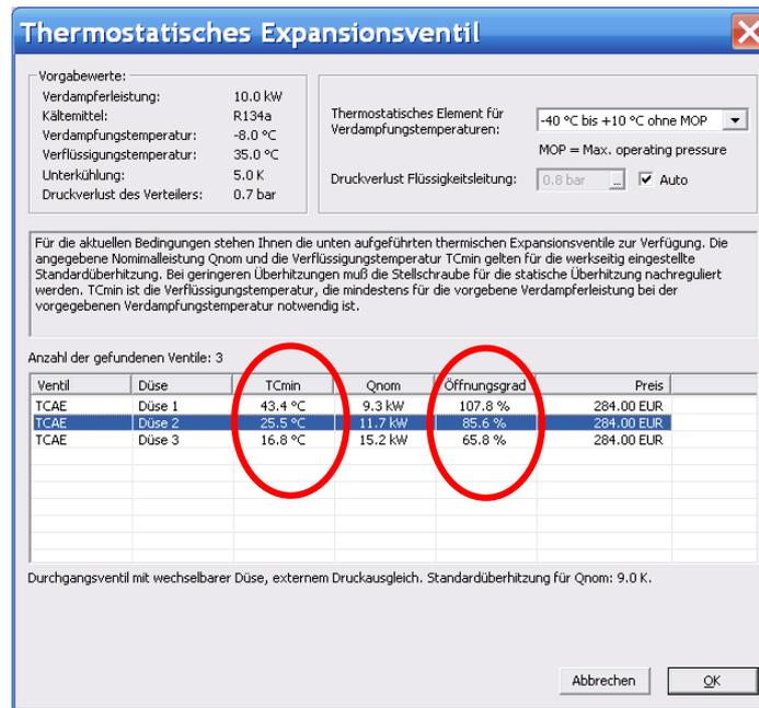
**Figure 5:** Configuration module for thermostatic expansion valves in GPC
