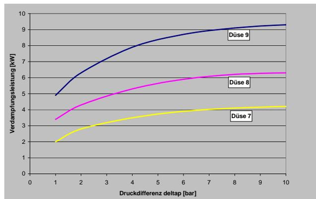
Figure 3: Refrigeration capacity of three different thermal expansion valves
