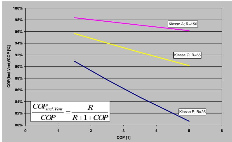
**Figure 8:** Percentage reduction of COP if the fan power is taken into account in relation to the energy efficiency class of a condenser
