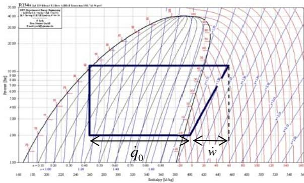
Figure 1: Single-stage refrigerant system
