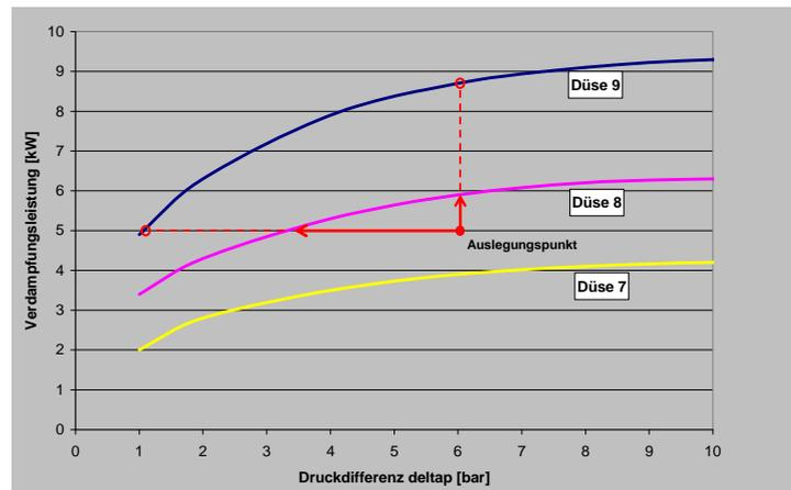
**Figure 4:** Configuration of thermal expansion valve and minimum permitted pressure difference
