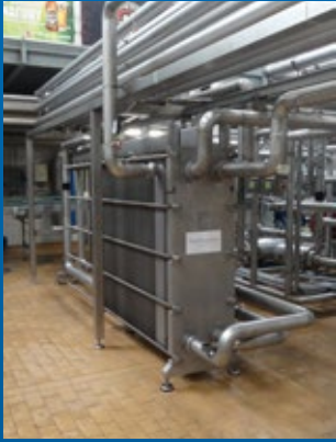
▲ A thermowave TL 500 FCGV unit, which boasts approx. 93 % heat recovery, is used as a pasteuriser for the high-temperature, short-time (HTST) flash pasteurisation of the beer for 15 to 30 seconds.
